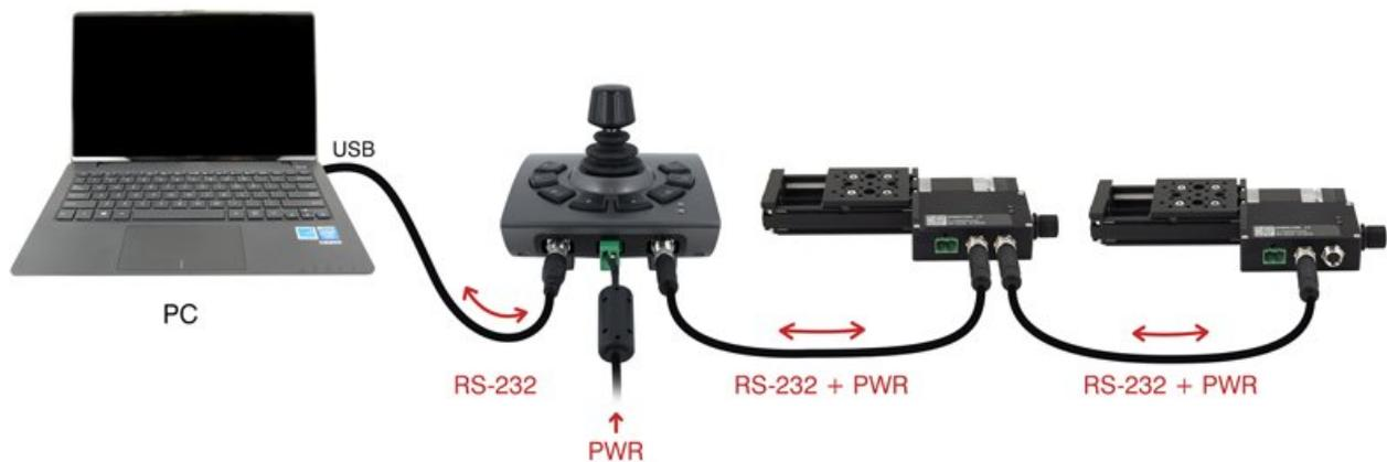
To daisy-chain X-Series devices with T-Series and A-Series devices:
