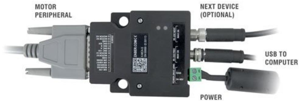
NOTE: Ensure no motors are connected to the controller before applying power for the first time. It is important that the controller is set to control the correct peripheral ID in order to avoid sending too much current to the motor. We try to set controllers for the peripherals they ship with, but it's good to check that they are correct, especially if you receive multiple peripherals of different models.
